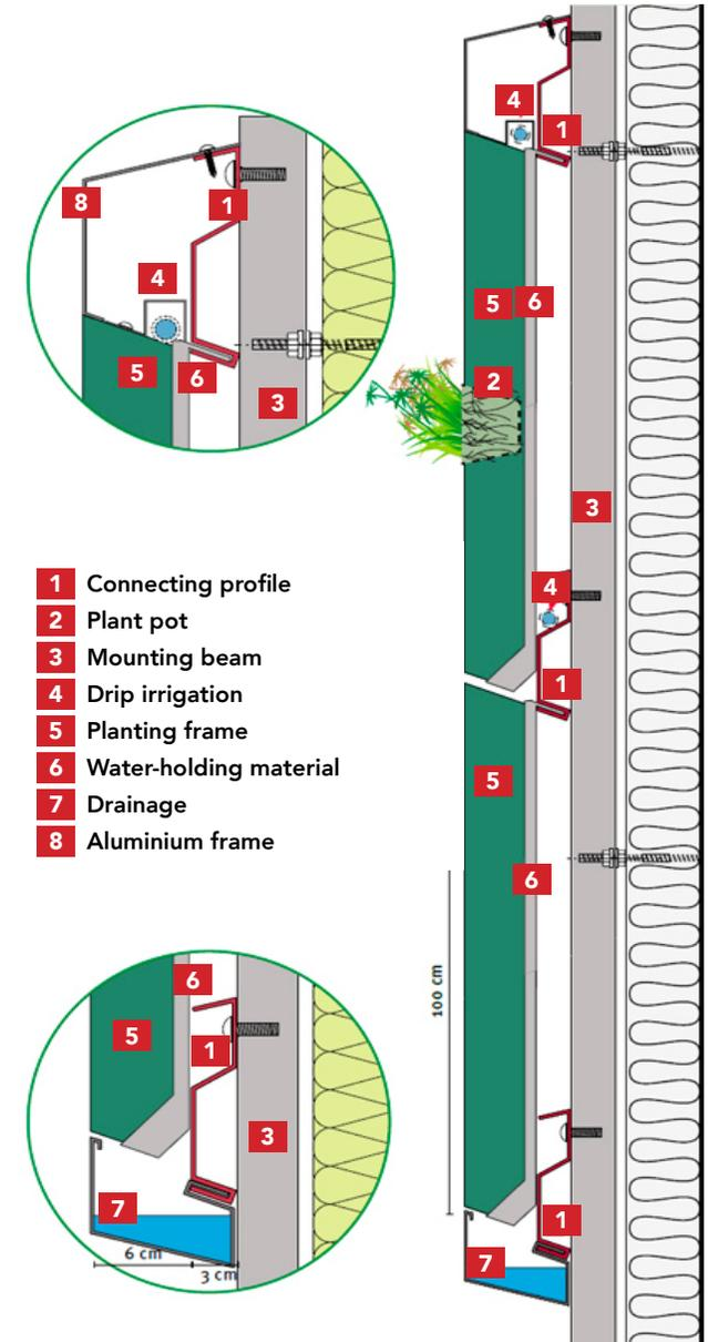
Figure 1. Structure of plant cassettes on the outside of an existing wall. (Source: Optigreen)
